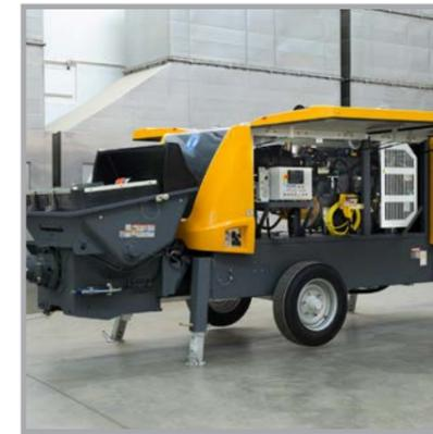
Swing doors provide easy access and protection from the weather
