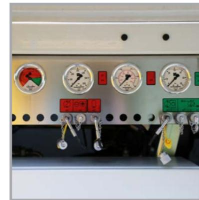
Mini measuring panel: hydraulic measuring points read from a central point
